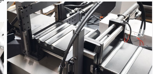
The full-travel vice on the feeder unit is equipped with two stable guide shafts; during travel, it opens on both sides to compensate possible unevenness of the material
